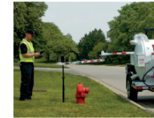
ERV-750 easily reaches any curbside valve box or hydrant within 13ft of the mount.
