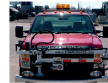
High stack version of the ERV-750 is available for bumper mounting.
