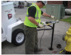
Highly portable handheld design allows operation of valves from 6-60in
